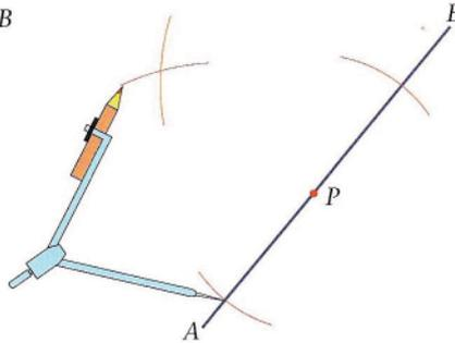
Join the point where the arcs cross to P. This line is perpendicular to AB at P.
