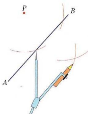
Join the points where the arcs cross to  $P$ . This is the line perpendicular from  $P$  to  $AB$ .
