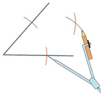
Join the point where the arcs cross to the vertex of the angle. This line is the bisector of the angle.
